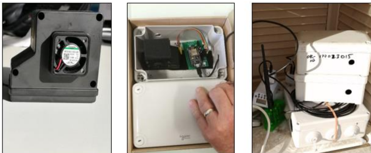
Figure 6 - Detail of one Alphasenses OPC-N3 sensors (left), detail of IRISA packaging (right) and two OPC-N3 in their box at Laënnec station (center)
