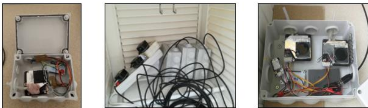
Figure 4 - Detail of one initial SDS011 sensor box (left), three of them in the meteorological shelter at Laënnec station (center), New experimental package (right) with two associated sensors to be able to evaluate bias
