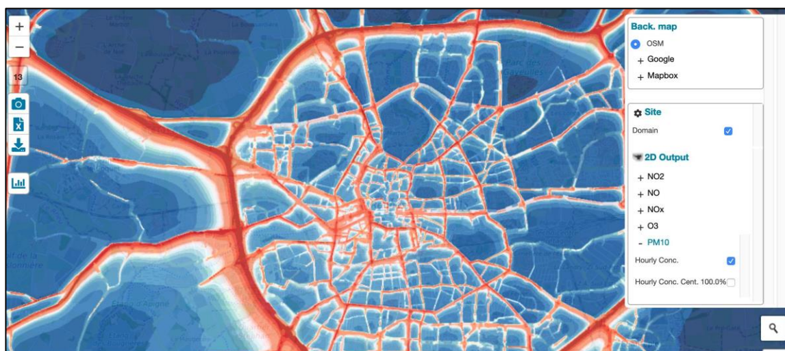
Figure 11: Concentration map obtained from SIRANE outputs and post processed through ATL. Map data for concentration can also be integrated in third party tools using AWMS API.
